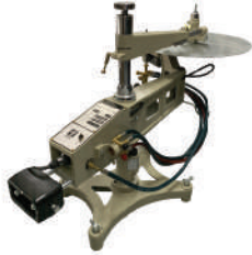
Profile Gas Cutting Machine TG2-150 Cutting Thickness : 6 - 100mm Diameter of Circle Cutting : 20 - 600mm Max. Size of Cutting Square : 500 x 500mm
